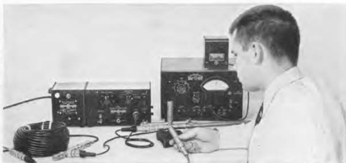
Figure 6. Unit Klystron Oscillator and Type 874 Coaxial equipment set up for the measurement of cable attenuation at 3000 megacycles.
