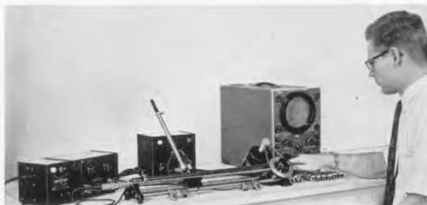
Figure 7. Unit Klystron Oscillator and Type 874-LBA Slotted Line with Motor Drive, set up for measurements of standing-wave ratio on coaxial attenuators.
