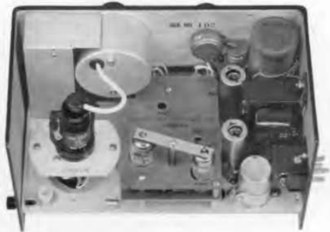
Figure 3. Top view of the oscillator with shield cover removed, showing the klystron tube.
